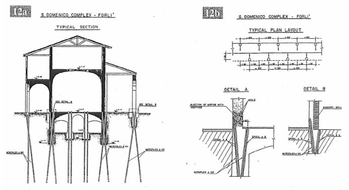
Different solutions can be adopted in case of steel reinforced concrete existing foundations.
