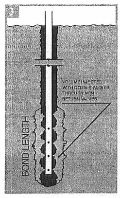
The ultimate bearing capacity of micropiles "Qu" given by lateral friction on bond length can be estimated as follow:
